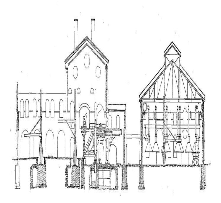
$Fig.~4. \\ -Section~of~Bessemer~House~and~Repair~Shop~Along~A~B.$
