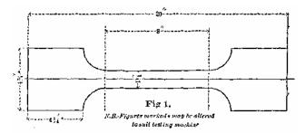
In the original specifications, it will be observed by reference to the above rules, that plates of only 58,000 pounds tensile strength might pass, provided the average of all the test-pieces was 60,000 pounds, or over; but, in the amended specifications we were not
