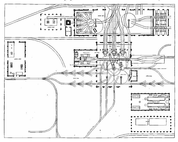
${\it Fig.~I.--General~Plan~of~Bessemer~Plant.}$  The Bessemer Plant of the North Chicago rolling mill company, at south chicago.
