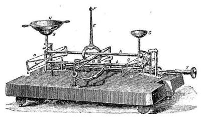
A. A, Parallel compound beam. B. Immovable centre frame, tarrying Index and beam. C. C. Movable frames carrying the pans. D. D. D, Stretched gold wires over the frames, acting as central and terminal pivots. M. Index. F. Weight for the purpose of elevating (he centre of gravity, (t. G. Cups for pans. II. II. I'ans, I. Arrest. A". A". Support to receive the weight of the scale when not in use.
