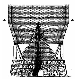
bosh, and 15½ feet, 17 feet and 18| feet high. The material required for this form of roaster closely approximates what is demanded for one of similar size of the pattern shown on Plate I less the cone and chimney.
