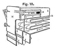
By opening the door, H, a scraper can be pushed through the gaschannels, and the burner fully cleaned in two minutes. The gaspassages are made larger than necessary when clean, to allow for some collection of flue-dirt.
