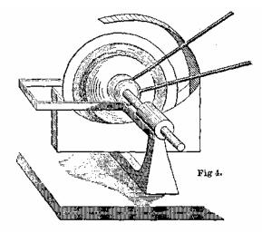
corundum or diamond-dust and cotton-seed oil. The cotton-seed oil with the cutting material adheres to the periphery of the saw, and as the saw comes in contact with a piece of iridium it gradually does the work. Cotton-seed oil is preferred for this purpose to any other oil, on account of its viscosity.
