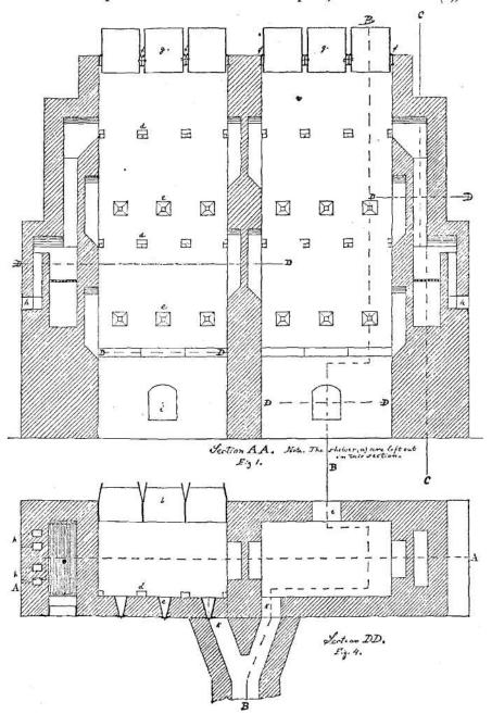
is located near the base of the kiln, but its hot gases enter below the top row of shelves, and move downward, finally escaping through the flue(k), which is connected with a chimney. Such an arrangement is made for very good reasons. If the fire entered below the bottom row of shelves, which are filled with dry and hot ore, a careless laborer might overheat and warp them by too heavy firing. As
